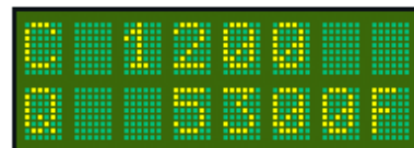
Adjusted encoder altitude for local QNH or BARO setting
